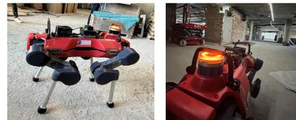
Figure 1: the Anymal robot setup used for data collection. The dataset was obtained over 4 stories of an ongoing construction project. It contains images of varying brightness, with a large amount of clutter and obstacles.
