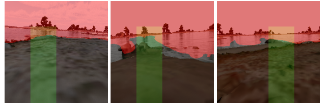
Figure 5. Three traversability segmentations and heuristic selections with water in the vicinity. The two on the right exhibit the peninsula effect.
