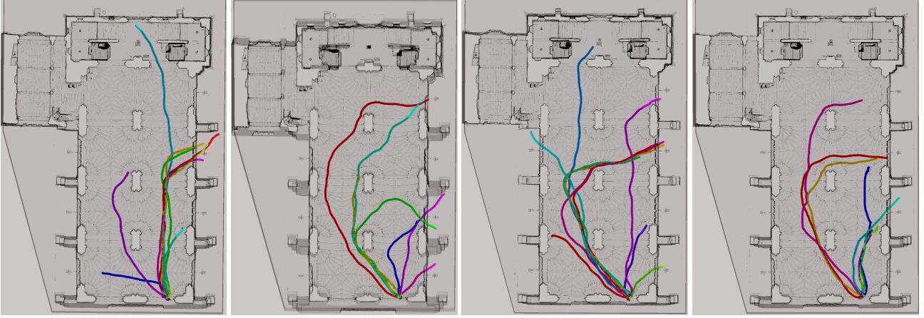
Figure 2. The four primary heuristics we tested out on our traversability signals rolled out ten times each on the Lincoln Inn Chapel Undercroft environment. Leftmost: Columns. Center left: Octants. Center right: Bottom-Heavy Octant. Rightmost: Bottom-Heavy Pairwise Octant. See Section 6 for more information on the right turning bias present in these rollouts.
